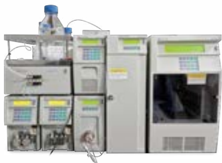
HPLC with High-pressure 6-way Switching Valve-UVD
